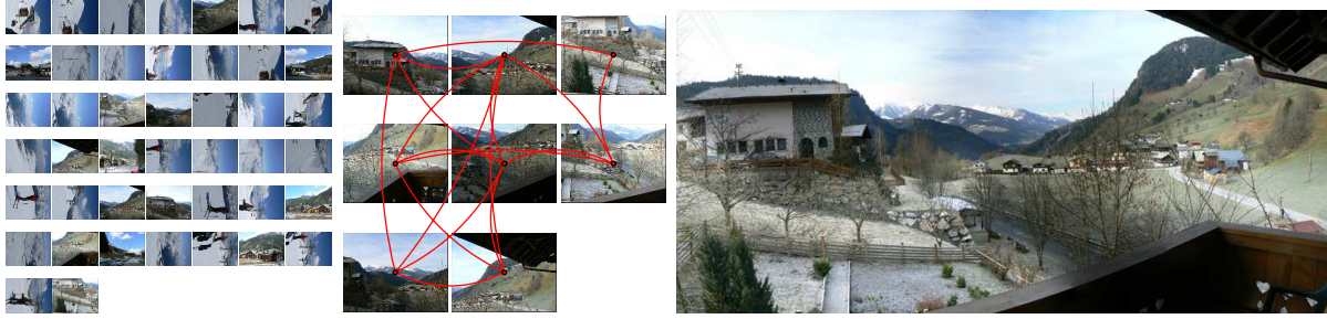
Figure 2: An unordered set of images with 3 panoramas on the left, matched images from one of panoramas in the middle and stitched panorama on the right.
