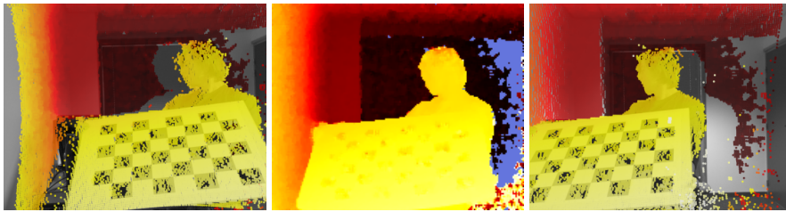
Fig. 4.1 The central panel shows a range image, colour-coded according to depth (the blue region is beyond the far-limit of the device). The left and right cameras were aligned to the ToF system, using the methods described here. Each 3-D range-pixel is reprojected into the high-resolution left and right images (untinted regions were occluded, or otherwise missing, from the range images). Note the large difference between the binocular views, which would be problematic for dense stereo-matching algorithms. It can also be seen that the ToF information is noisy, and of low resolution.
