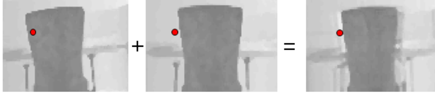
Fig. 1.5 TOF depth motion-blur due to movement of the target object.
