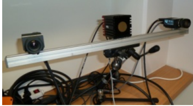
(a) A ToF-stereo setup
