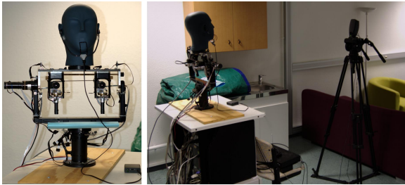
Figure 3: A binaural head is placed onto an agile device that can perform precise and reproducible pan and tilt motions (left). The emitter (a loud-speaker) is placed in front of the robot head at approximately 2.7 meters (right).
