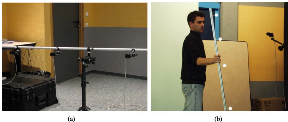
Fig. 2 (a): Partial view of a 30-camera setup. (b): The calibration data are gathered by moving a one-dimensional object in the common field of view of the cameras
