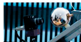
Fig. 15. Homemade catadioptric camera built from a Basler A201bc camera with a Fujinon 12.5 mm lens pointed at a Christmas ornament representing a roughly spherical mirror.
