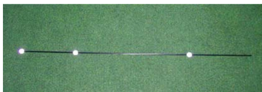
Fig. 2 Single calibration wand used for ‘wand dance’
