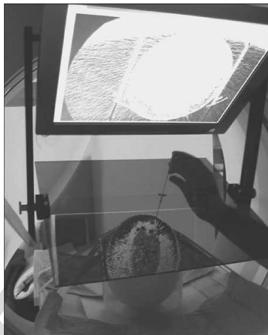
Fig. 2. Needle insertion in a head-phantom. The CT image of the water melon is floating inside the phantom.
