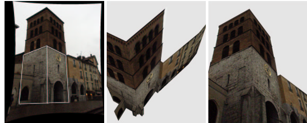
Figure 4: Notre-Dame square scene in Grenoble, France: the single original image (radial image distortion was corrected off-line) and screen-shots of the 3D model.
