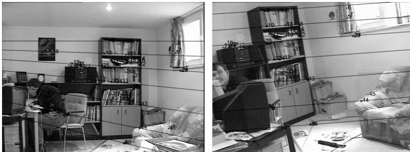
Fig. 12. This figure shows the epipolar geometry as computed with the matching and estimation method described in this paper. Notice the large discrepancy in the viewpoints associated with the two images. The matcher seems to give advantage to collections of coplanar points.
