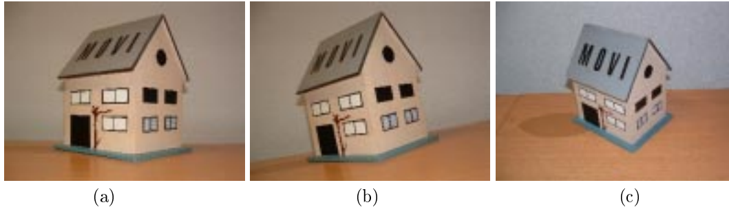
Figure 3: Examples of singular and non-singular configurations for calibration based on a parallelepiped with three right angles; (a) The parallelepiped's vertical edge is parallel to the camera's y -axis; this configuration is singular if the camera aspect ratio and principal point are not given (cf. cases B-3-0 and C-3-0 in table 3). (b) The parallelepiped's vertical edge is parallel to the image plane; this configuration is singular if the camera's principal point is not given (case B-3-0 in table 3). (c) A rotation of the camera as shown here removes the singularities of (a) and (b).
