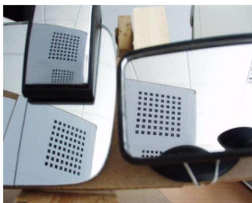
3 Mirror + pinhole camera (non-central scenario)
