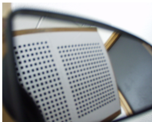
convex mirror + pinhole camera
