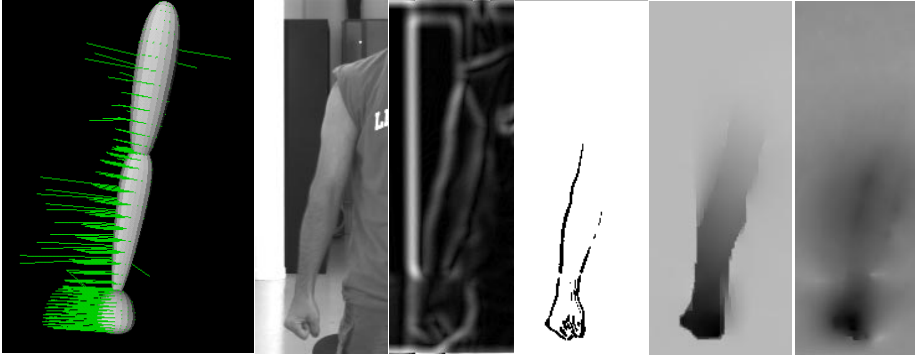
Figure 3.2: A view of an arm model (a), and examples of our robust low-level feature extraction: original image (b), intensity edge-energy (c), motion boundaries (d), robust flow field in horizontal (e) and vertical direction (f).
