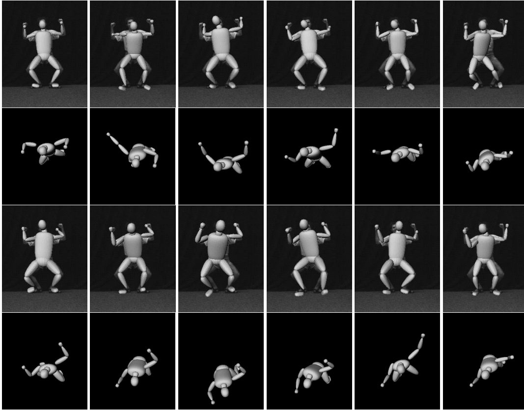
Figure 6.6: Human poses sampled using hyperdynamics on a cost surface based on given model-to-image joint correspondences, seen from the camera viewpoint and from above. Hyperdynamics finds a variety of different poses including well separated reflective ambiguities (which, as expected, all look similar from the camera viewpoint). In contrast, standard stochastic dynamics (on the same underlying cost surface with identical parameters) essentially remains trapped in the original starting mode even after 8000 simulation steps (fig. 6.8).
