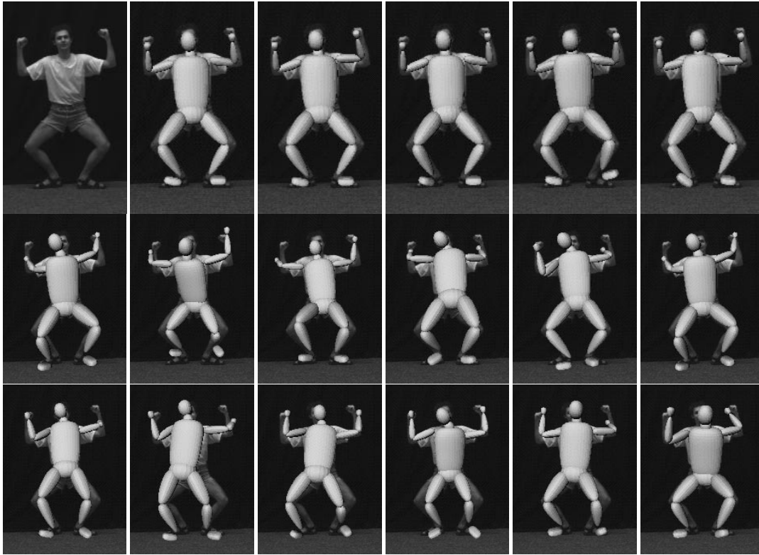
Figure 5.6: Minima of image-based cost functions. Top row: contour and optical flow likelihood. Middle and bottom rows: silhouette and edge likelihood. The model is initialized in one minimum (first row, second figure), and search trajectories for other minima (along different principal curvature directions) are initiated from there. The other figures show some other minima found, that correspond to incorrect contour assignments or to configurations where the intensity robustifiers turn off (see text).
