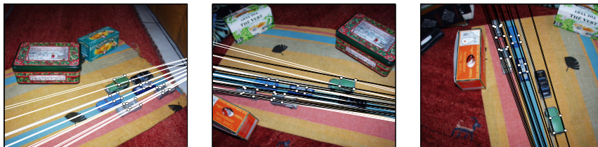
Figure 4: Motion line pencils estimated using two-view projective bundle adjustment. For the middle image, we compute the motion line pencils with respect to two C-tensors (with the first and with the third images). Note the significant discrepancy between them. This discrepancy will be eliminated by a consistent parameterization of the multiple-view case, see §3.2. Note also that points lying on the overtaking car have been discarded as outliers.
