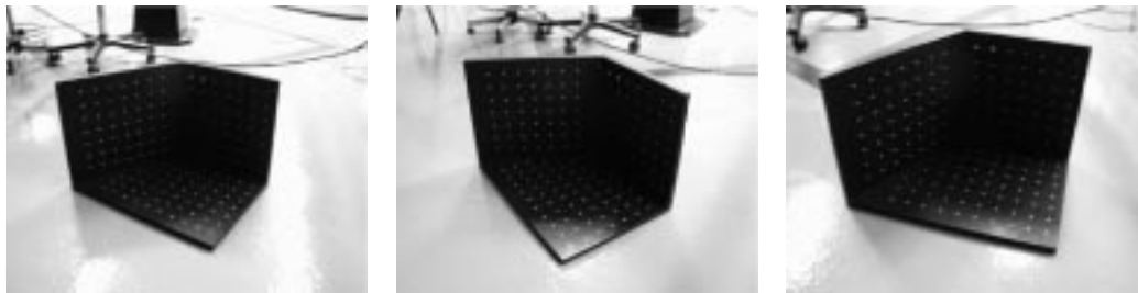
Figure 15: Three images of a calibration grid amongst the 7 used in the experiment.
