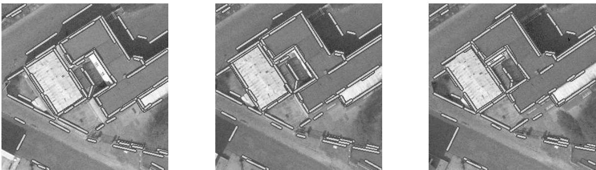
Figure 23: Three view line matching II: These images are a sub-part ( 600 \times 600 pixels) of those in figure 21. There are 248/236/212 detected line segments and 89 lines are matched, all of which are correct.
