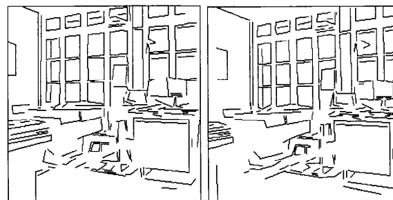
Fig. 16. The matched lines for the first image pair.
